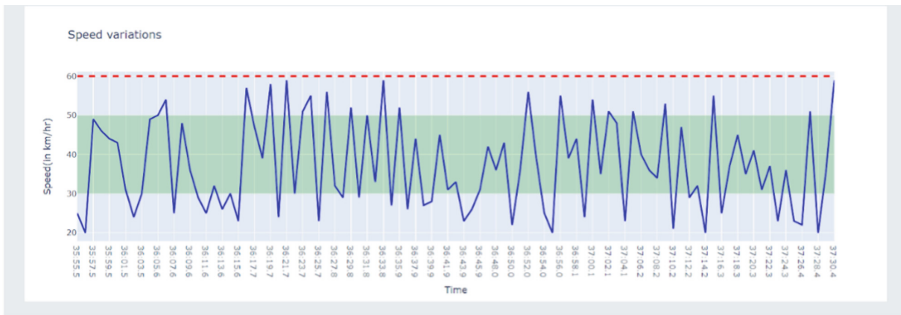
Fig. 9. The speed variations datapoints are plotted and ideal speed expected to be maintained is within the green box i.e. between 30–50 km/h.
