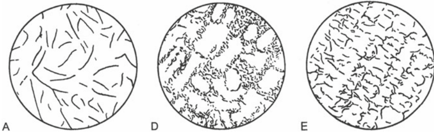
Fig. 14.3 Graphite arrangements A (left), D (middle) and E (right). Excerpt from: directional series diagrams for arrangement of graphite in cast iron according to DIN EN ISO 945-1:2019
