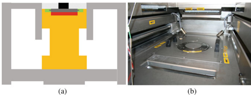
Fig. 3.10 Heated building chamber a schema b photo of front view
