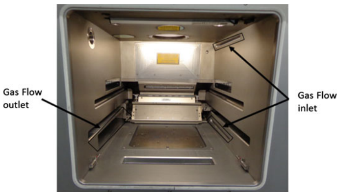
Fig. 3.8 Front view to building chamber
