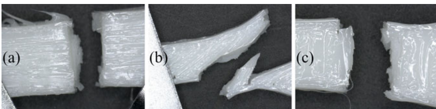
Fig. 9.5 Break pattern of samples with a 0°, b 45° and c 90° orientation
