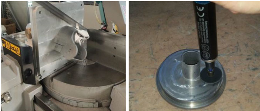
Fig. 3.12 Removing support structures: from platform (left) from AM-part (right)
