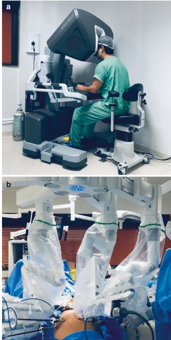
Fig. 25.1 DaVinci™ robotic operating system. (a) Surgeon console where the movements are performed and sent to the unit attached to the patient. (b) Robotic unit that performs the surgeon's movements, consisting of articulated robotic arms with instruments introduced into trocars located in the abdominal wall under supervision of an assistant. (Photo: with permission from Ricardo Miyaoka, 2021)
