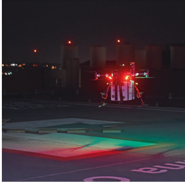
Fig. 23.1 LG-1000 four-arm octocopter drone carrying the first donor kidney for human transplant landing at University of Maryland Medical Center, April 2019
