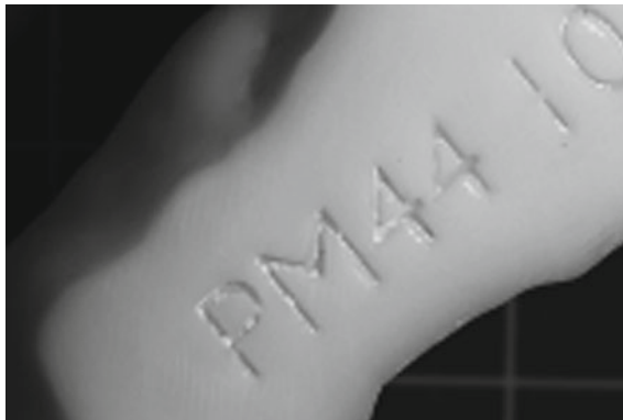
Fig 5.23 Shows unique identifier debossed for audit trail of evidence [19]. Licensed by Springer Nature, License Number 5280780965869
