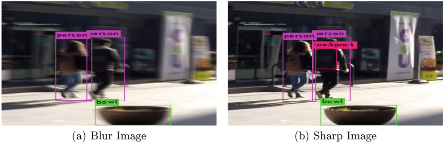
Fig. 1. The figure shows object detection on images becomes easy after deblurring using FMD-cGAN. YOLO [2] object detection on the (a) blurry picture and on the (b) sharp picture from the GoPro dataset [3]
