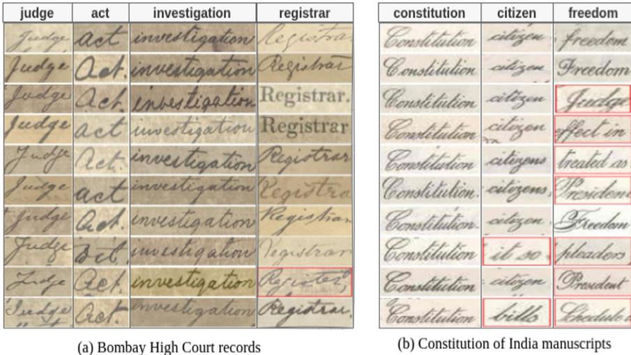
Fig. 4. Top-10 qualitative search results from collections: BHC records and CoI manuscript. Queries are shown at the top and incorrect retrievals are highlighted in red. Querying is done in QbS setting. Poor image quality of the collections is also shown here. (Color figure online)
