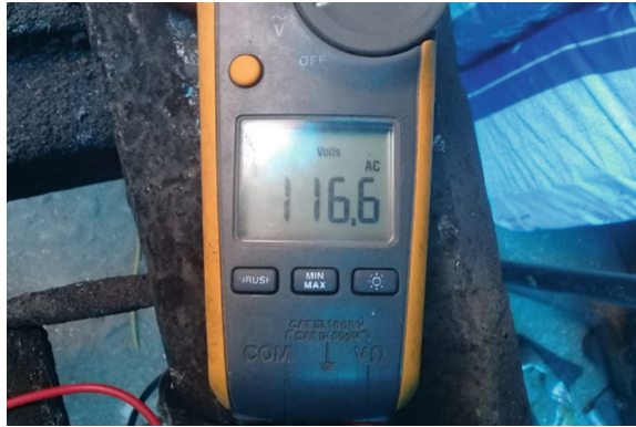
Fig. 8. Measurement obtained by the commercial multimeter, of the voltage supplied in the premises (Metal mechanics the locksmith).
