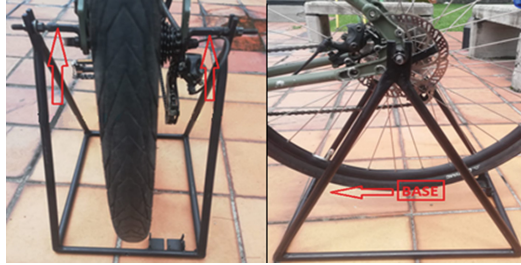
Fig. 5. Base of the dynamo.
