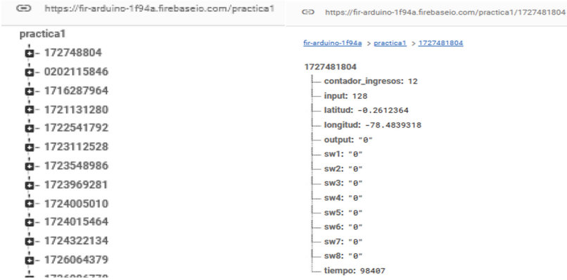
Fig. 7. Structure of practice 1 storage in the cloud and activity registered by user
