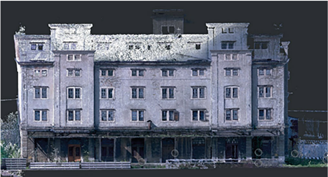
Fig. 7 Warehouse 20's points clouds (Recap PRO)
