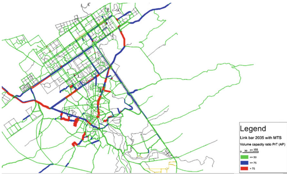
Fig. 3 Volume capacity ratios of city road network with MTS (with BRT Lines)
