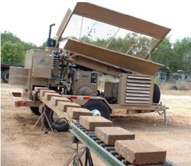
Fig. 3 Production and use of bricks from local materials at sites. Source Al Saeed and Jamal Abdul Ghani (2017)
