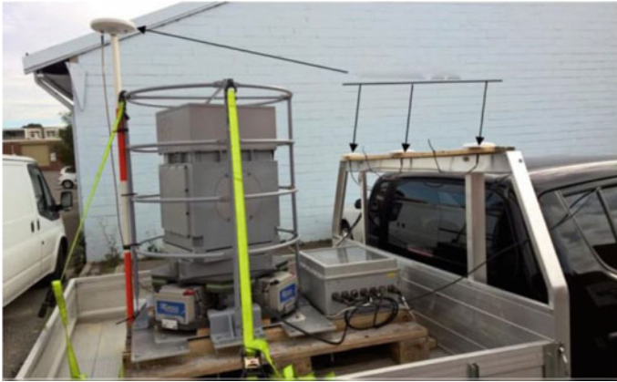
Fig. 4.21 GT-2AQ gravimeter with Javad QUATTRO-G3D GNSS antennas in the cargo tray of a pickup truck
