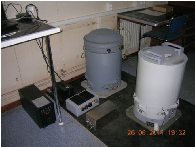
Fig. 4.5 Chekan-AM ( left ) and Shelf-E ( right ) gravimeters onboard the Akademik Fedorov research vessel
