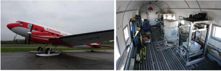
Fig. 4.24 Bastler aircraft and GT-2AP gravimeter in the aircraft cabin
