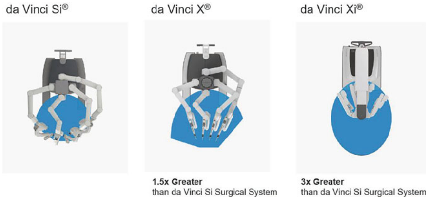
Fig. 10.3 Worspace comparison between the three latest da Vinci Surgical System generations. Credit Intuitive Surgical, Inc.
