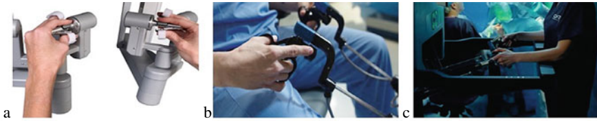
Fig. 9.2 Different types of grips for master controllers. a pinch grip in da Vinci [7]. b Power grip in Senhance [37]. c power grip (joystick) in Versius [38]
