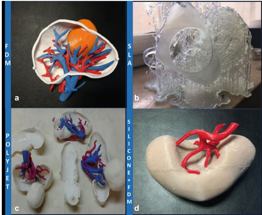
Fig. 12.2 3D printing technologies: a Fused Deposition Modeling (FDM); b Stereolithography (SLA); c Multi-material Plastic Jetting (Polyjet); d Silicone mold pouring combined with FDM printing
