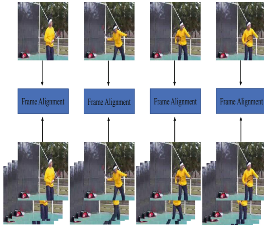
Fig. 2. Frame Alignment compares the sampled frames of the Sparse pathway and the Dense pathway. In this way, the consistency of the processing information of the Sparse pathway and the Dense pathway can be guaranteed. While ensuring the diversity of network input information, it also reduces the computational cost of the Dense pathway.
