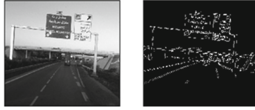
Fig. 4. After edge detection Canny process in ROI.
