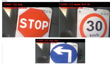
Fig. 10. Example of real-time sign detection.
