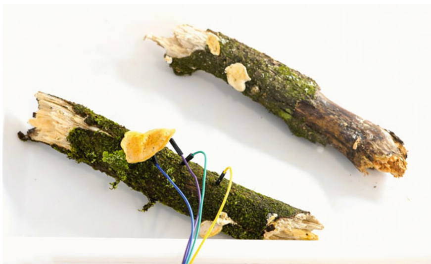
Fig. 8 Reading electromyceliograms, the electronic signaling of mycelia (Cesar & Lois 2022)
