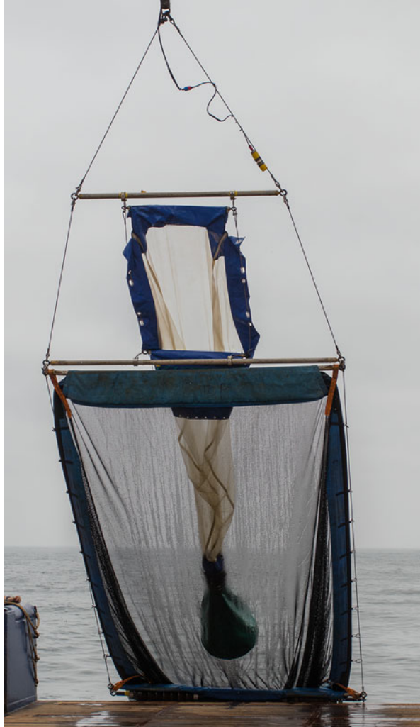
Fig. 11.11 Mesopelagic fishes, large crustaceans and gelatinous plankton were collected using a Rectangular Midwater Trawl (RMT 8)
