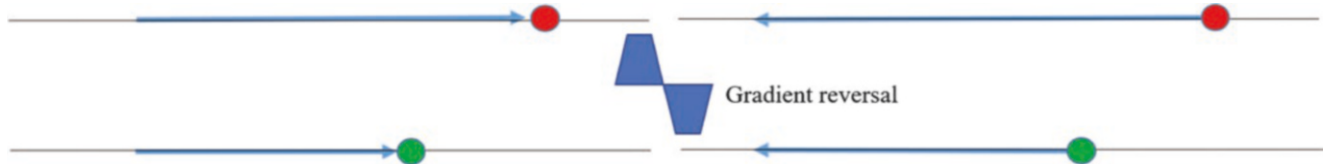
Fig. 20.7 Gradient echo formation diagram. Two spins are dephasing at different rates prior to rephasing readout. The gradient payout is analogous to two runners turning and running back to the “start line” to create an echo
