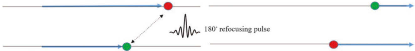
Fig. 20.3 A representation of what spins experience after the spin-echo refocusing pulse. The pulse is analogous to two runners swapping lanes such that they arrive at the “finish line” in unison, thereby creating an echo
