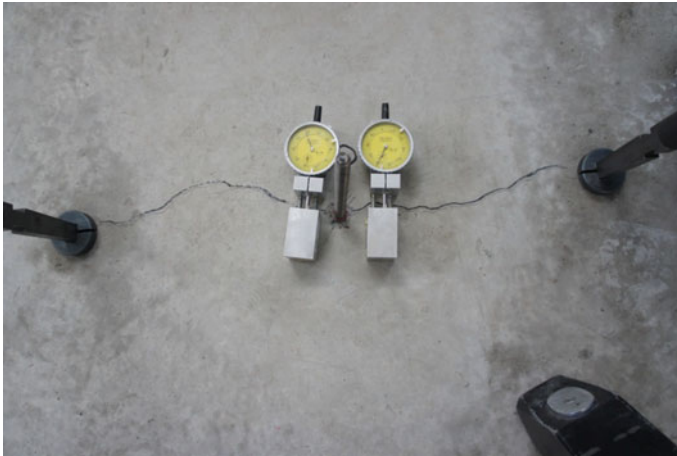
Fig. 1 Control of crack width
