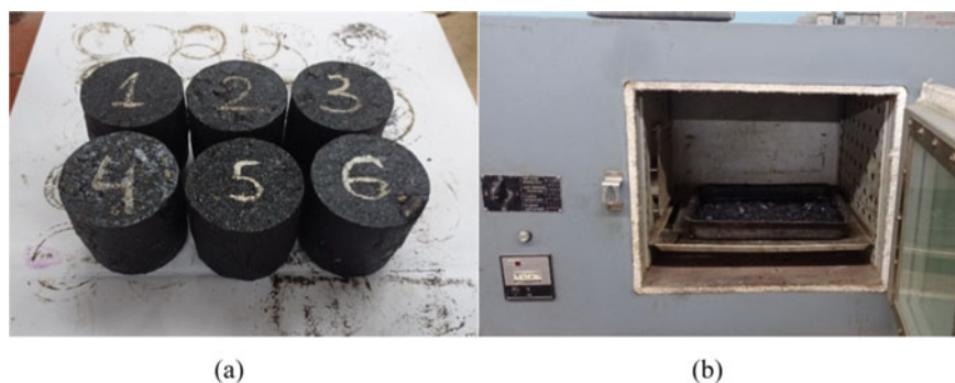
Fig. 1 a – The standard cylindrical specimens size of 71.4 mm. b – The Bitumen-limestone crushed stone on metal trays in ventilated thermal furnace
