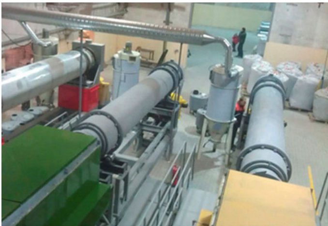
Fig. 1 General view of the experimental plant for the production of foam granulates
