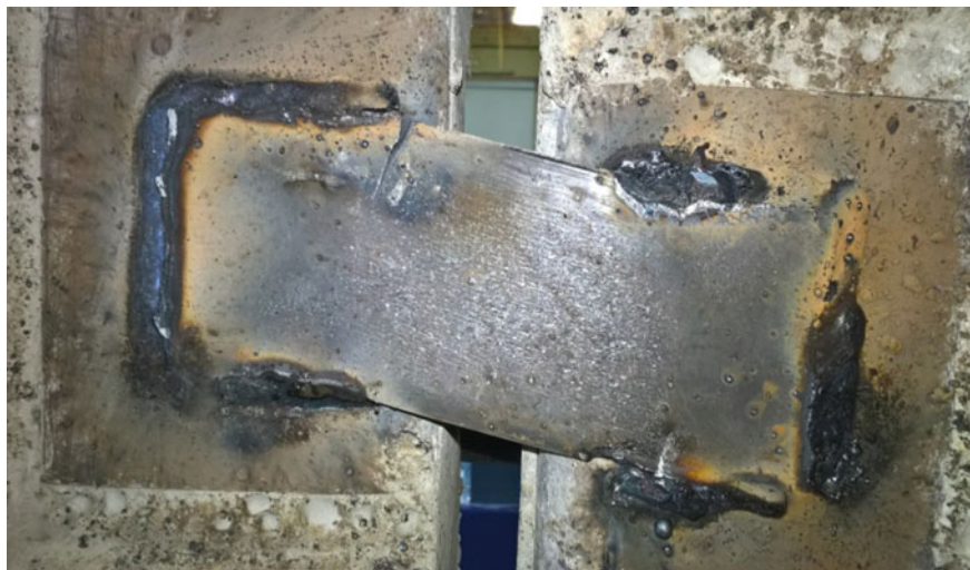
Fig. 1 Destruction of the connecting plate during shear
