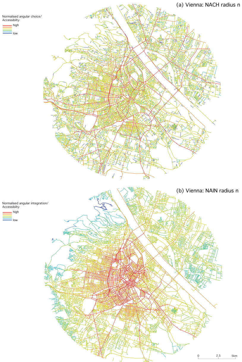
Fig. 1. City-wide configurational analysis of Vienna's street network: (a) NACH radius n, (b) NAIN radius n [6] (p. 526), [12] (p.77). (Color figure online)
