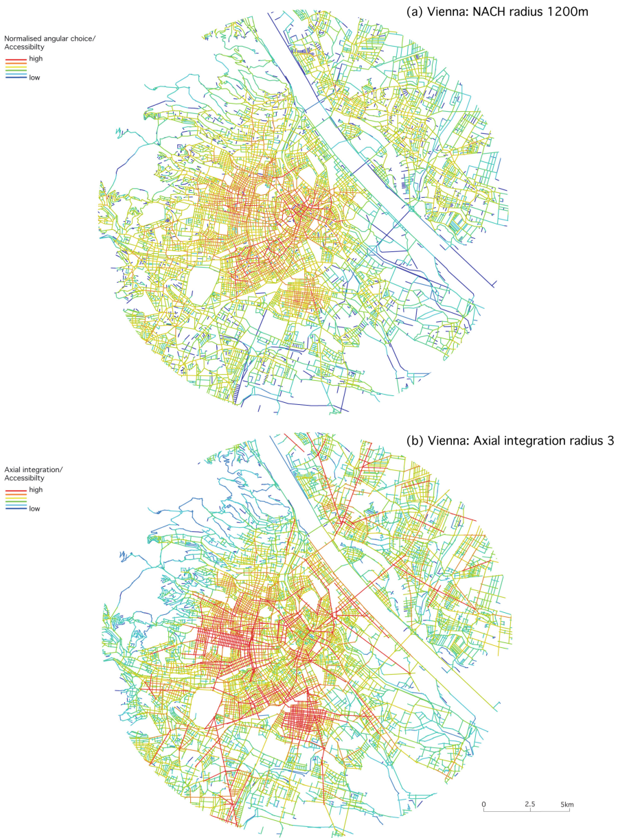
Fig. 2. Local configurational analysis of Vienna's street network: (a) NACH radius 1200 m, (b) Integration radius 3 (axial map credited to Sebastian Zeddel; model computed by the authors)
