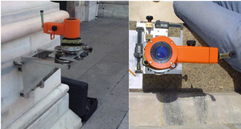
Fig. 11. Measurements of tilt variations using an optical plumb installed on the façade and apse of the Duomo. The configuration on the left allows the connection of a vertical surface. The figure on the right shows the installation on a permanent reference on the floor.
