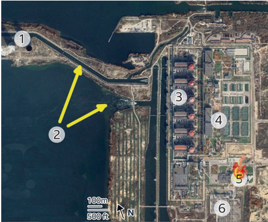
Photo 6 A satellite view of the site (source IAEA). 1: Air coolers (x2); 2: Channels for the supply and discharge of cooling water (cold source); the channels run along the 6 plants; 3: The 6 WWERs, the rectangular buildings with red roofs perpendicular to the water supply channel for the condensers, correspond to the turbine buildings (engine room); the reactors are in the cylindrical buildings with red domes; 4: Spent fuel and radioactive waste storage area; 5: Training building where the fire started; 6: Power evacuation electrical lines station
