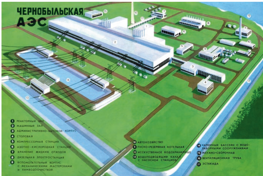
Fig. 4.1 An artist's drawing presenting an idyllic vision of the Chernobyl site from a 1978 presentation brochure. The turbine building (noted 2) is common to two twin plants. The two twin reactors are noted 1
