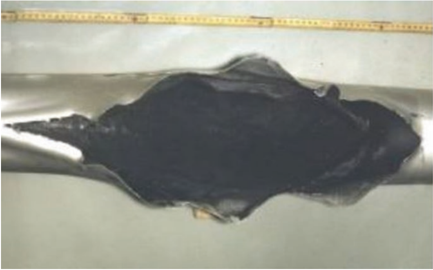
Photo 2.70 Impressive view of the cladding of fuel element 59. The cladding is completely torn
