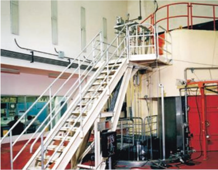
Photo 2.99 The RA-3 reactor whose main function is the production of medical isotopes such as metastable technetium 99
