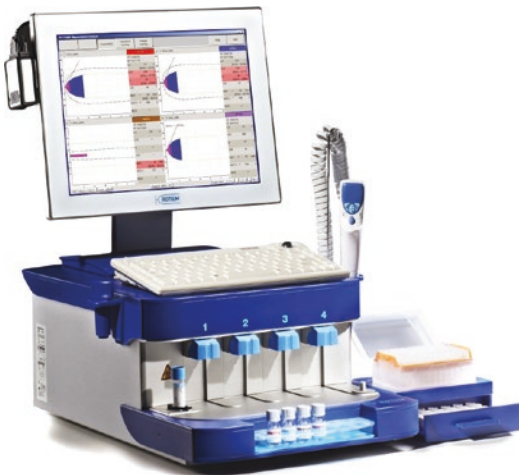
Fig. 5 Photograph of the ROTEM delta hemostasis analyzer. (Courtesy of Werfen, Barcelona, Spain)
