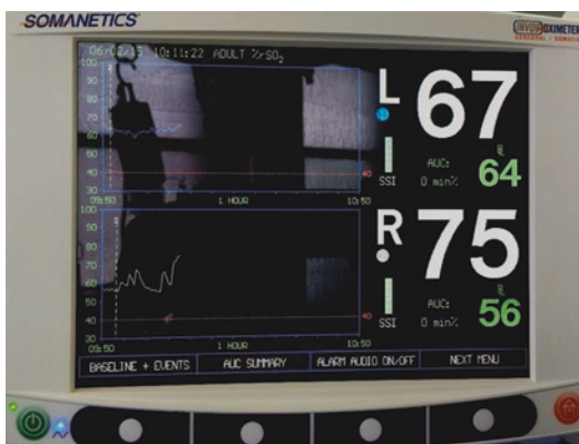
Fig. 2 Intraoperative bilateral NIRS for cerebral oxygenation monitoring. (Published with kind permission of © Medtronic, 2016. All Rights Reserved)
