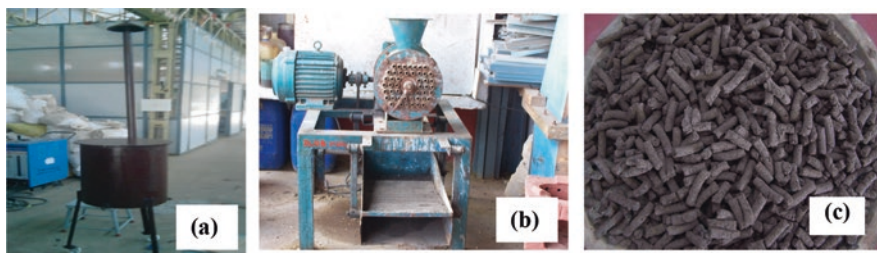
Fig. 4 TNAU developed (a) pyrolysis unit, (b) biomass, coal, and binder material pelletizer, and (c) manufactured pellets
