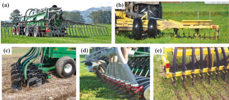
Fig. 11 Efficient liquid manure application. (a) Trailing hose. (b) Aeration. (c) Deep injection. (d) Shallow injection. (e) Trailing shoe. (Source: Anon., 2012a)
