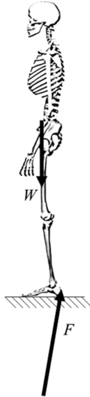
Fig. 3.5 Different free body diagrams under the same blast loading situation at time t = 0 . These demonstrate that the appropriate choice of a free body diagram can allow internal forces to be quantified
