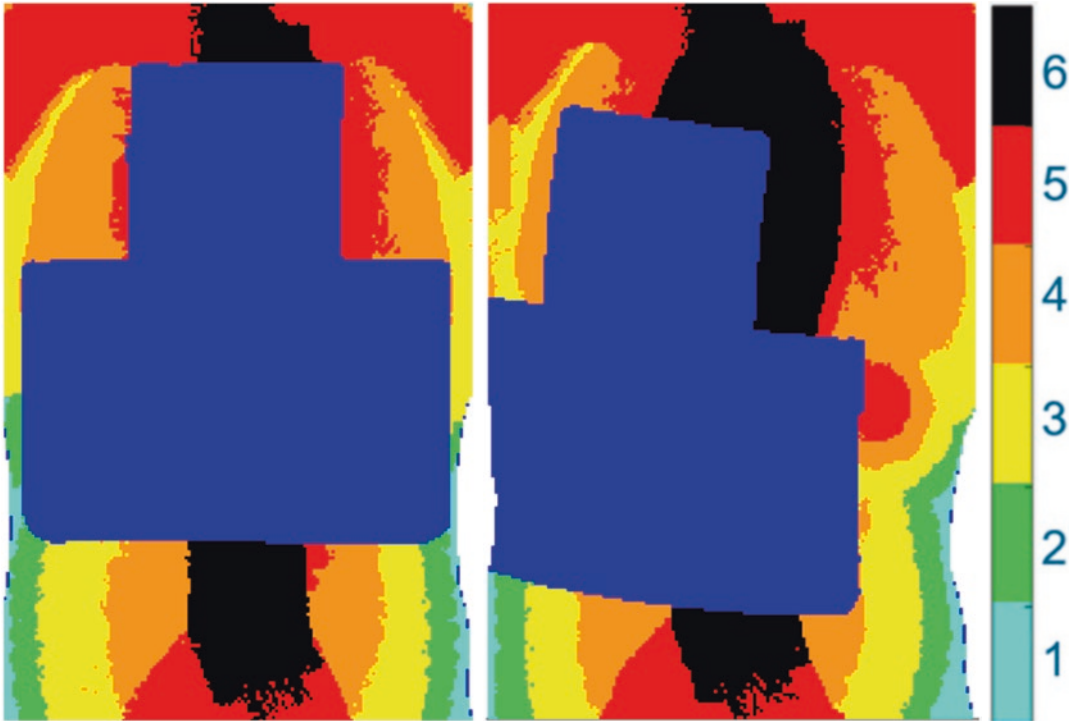
Fig. 37.8 Example of output from Weapon Target Interaction model. The blue area represents shot lines being stopped by the hard plates; the other colours correspond to Abbreviated Injury Scale 1–6 as shown on the right of the diagram
