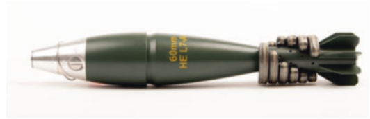
Fig. 8.2 A 60 mm mortar bomb showing the fuze, body and augmenting propelling charges around the tail unit
