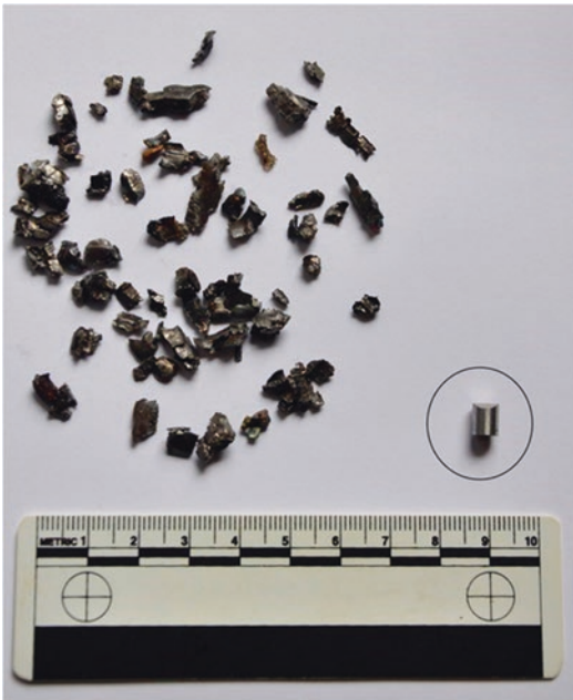
Fig. 35.4 Examples of actual fragments from a Mortar Bomb 81 mm HE L41 (left) and 1.1 g chisel nosed FSP (right; circled). Photograph: DJC
