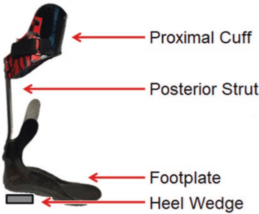
Fig. 42.2 Carbon fibre custom dynamic ankle foot orthosis (IDEO) consisting of a proximal cuff, carbon fibre posterior strut for energy storage and return, carbon fibre footplate to protect the foot and act as a lever, and heel wedge for alignment and cushioning
