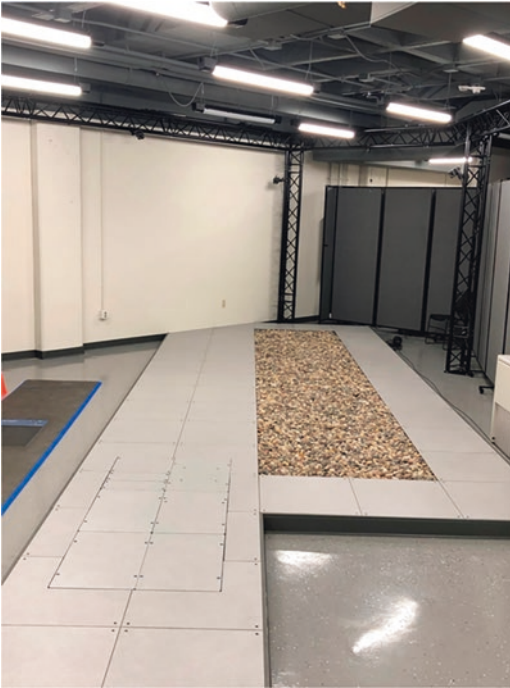
Fig. 42.5 Self-selected walking velocity can be measured using both flat level ground and uneven terrain as seen here. The time required to cross a specified distance is used to calculate the walking velocity
