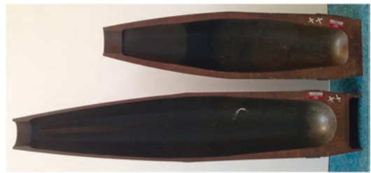
Fig. 8.4 Artillery shells showing the fuze cavity at the top and the differing thickness of the shell walls which on initiation of the explosive fill become fragments
