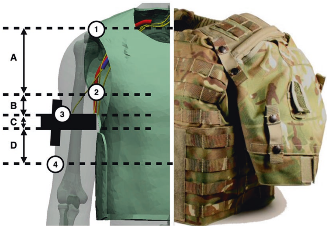
Fig. 37.13 A pictorial representation of how upper arm coverage was determined to optimise the VIRTUS brassard from the sum of distances (a–d). (1) Acromion pro-
