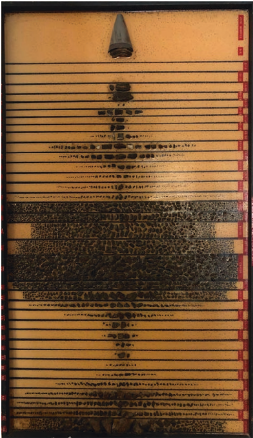
Fig. 8.5 The quantity and size of fragments resulting from initiation of a 105 mm artillery shell
