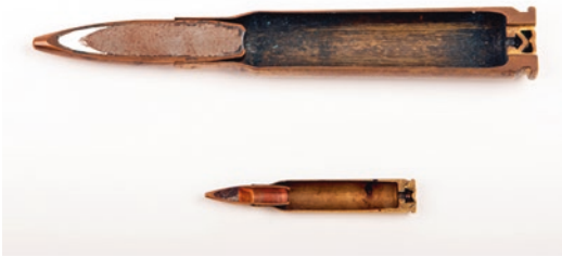
Fig. 8.1 A sectioned small arms round showing the bullet, the cartridge case and the percussion cap
