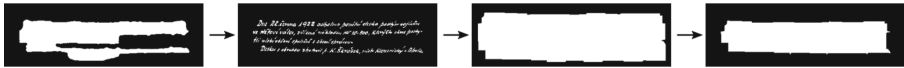
Fig. 10. Post-process example (from left: component from text mask prediction, masked binarised image, dilation, erosion).
