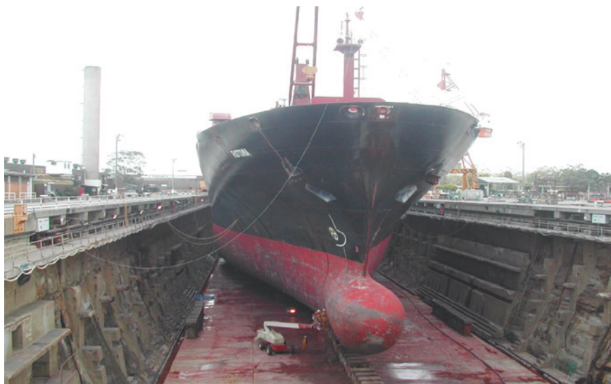
■ Figure 13.2 Stripping TBT-based antifoulant paint from a ship hull during drydocking for maintenance and repaint in the Port of Brisbane, Australia during the 1990s. After work completion the drydock was re-flooded, and paint debris accumulated on the dock floor was flushed into the river. Photo: M. Mortimer
