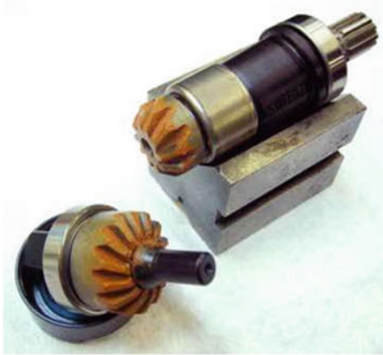
Figure 5: Contact pattern in geometrically-accurate spiral bevel gears in roll test.
