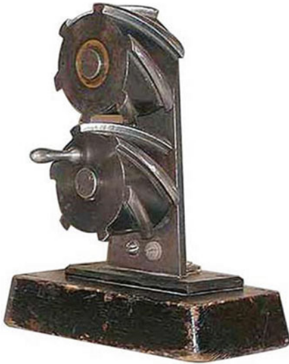
Figure 2: Rotationally-positive external parallel-axes gear pair (Pat. No. 163857, USSR, A Helical Gearing, /B.V. Shitikov, N.A. Bayazitov, Int. Cl. F06h, Filed: February 25, 1963, Published: July 22, 1964.).
