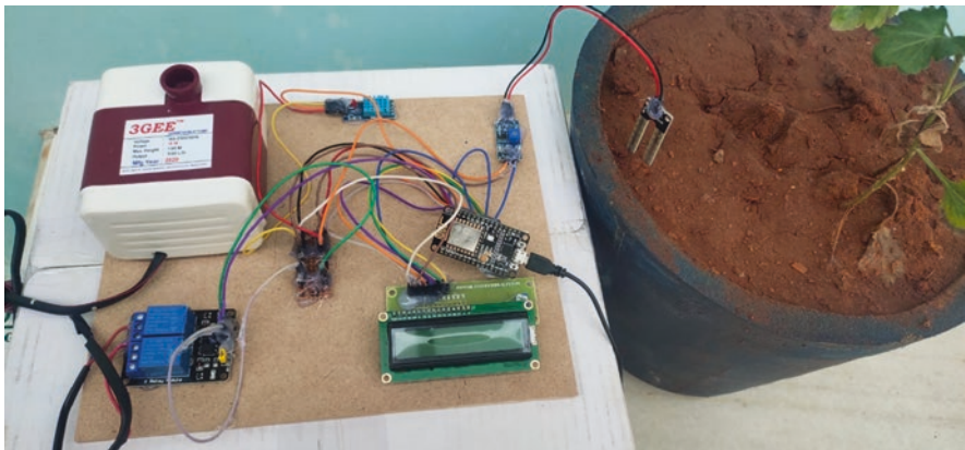
Fig. 5 Developed hardware module of irrigation model using IoT
