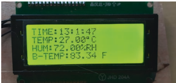
Fig. 14 Displaying the overall output on the LCD display
