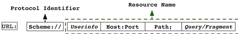
Fig. 2. Example of a URL. The protocol identifier and the resource name are separated by a colon and two forward slashes.
