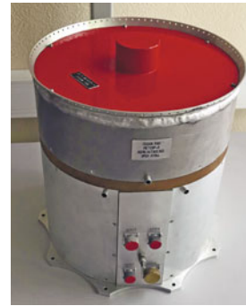
Fig. 36 The cosmic dust detector METEOR-L for the lunar orbiting spacecraft Luna-26
