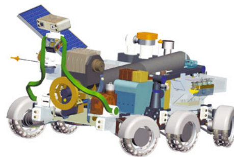
Fig. 38 The concept of a new generation heavy lunar rover “Robot-Geologist” with a drilling rig for carrying out geological and geophysical surveys on the Moon
