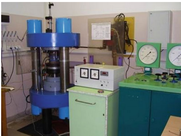
Fig. 10 Solid compression high-pressure apparatus for experiments up to 70 kbar and 1500–1700 °C
