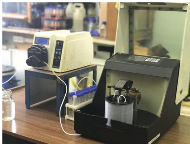
Fig. 25 Planetary centrifuge for separation of soluble components in a rotating coiled column
