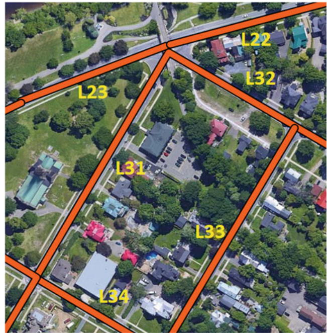
Fig. 3 Example of lanelets on a section of the surveyed area
