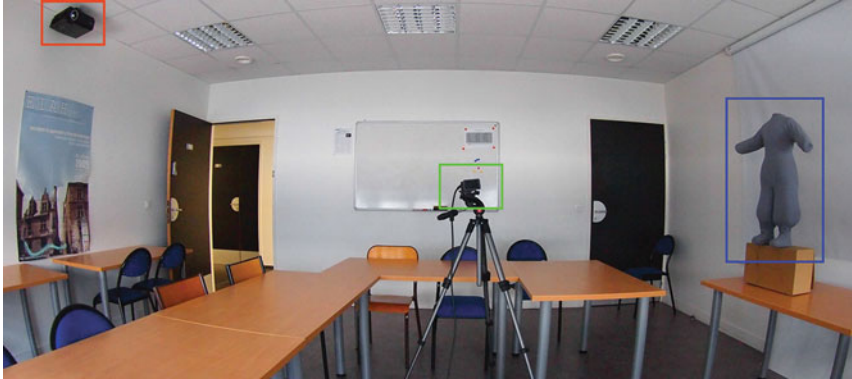
Fig. 6 Panoramic view of the hardware setup: the Kinect v2 RGBD camera (central green rectangle) is pointed to the puppet (right blue rectangle) on which the video-projector (left red rectangle) must project its suit
