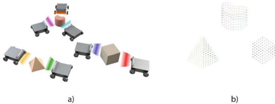
Fig. 16 Seven robots scanning three objects with the TVS (a) representation of seven robots scanning three objects (b) point cloud obtained by seven robots scanning three objects
