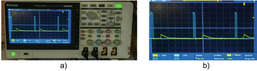
Fig. 11 Optocoupler and photosensor signals. (a) Oscilloscope used for signal visualization, (b) closer view of signals
