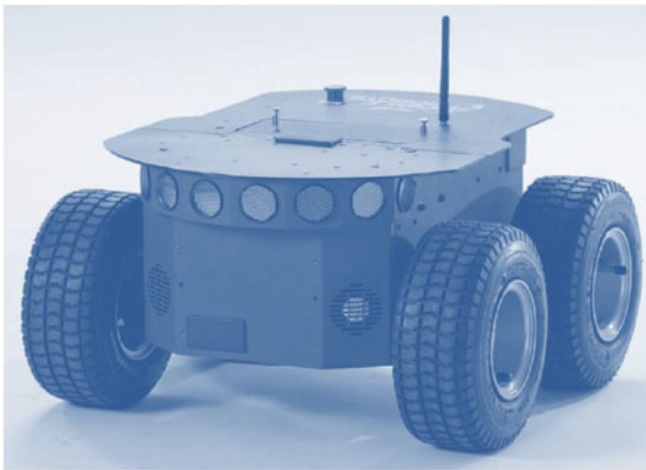
Fig. 6 Pioneer 3-AT research robot model
