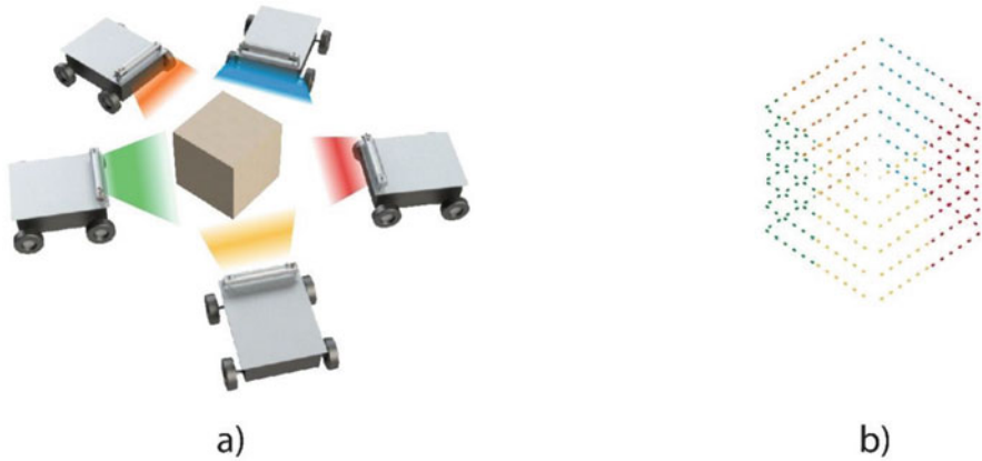
Fig. 13 Five robots scanning one object with the TVS (a) representation of five robots scanning one object (b) point cloud obtained by five robots scanning one object
