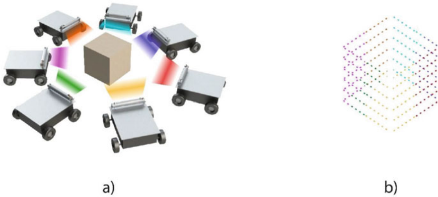
Fig. 15 Seven robots scanning one object with the TVS (a) representation of seven robots scanning one object (b) point cloud obtained by seven robots scanning one object
