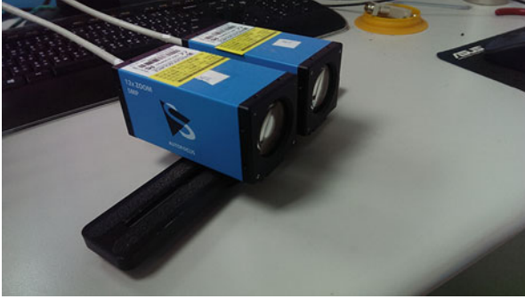
Fig. 10 Two DFK Z12GP031 cameras used in the experiments. The pixel size and original image resolution are 2.2 \mu\text{m} and 2592 \times 1944 , respectively
