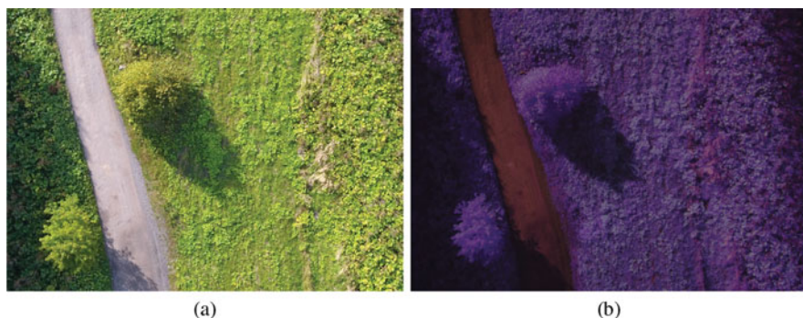
Fig. 3 Example of aerial imagery for (a) RGB camera and (b) multispectral camera
