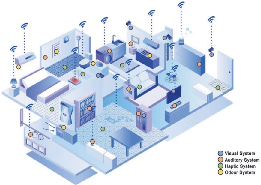
Fig. 9 Placement of four different types of perceptual systems in a two-bedroom apartment
