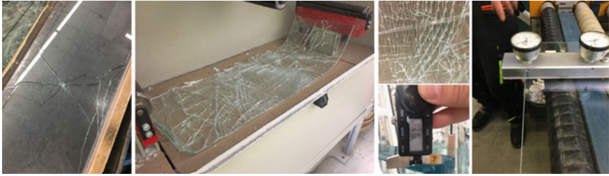
Fig. 8.20 Laboratory test on glass specimen (from left to right: fragmentation tests, edge offset measurement, local bow and roller wave measurement)
