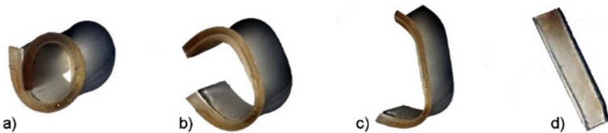
Fig. 10.3 Prototype A: Initial test of SMP responsiveness: a the deformed shape of a fabricated sample after applying heat and pressure, and the shape recovery process when re-applying heat for b 2 s, c 6 s, and d 8 s (Mansoori et al., 2019)
