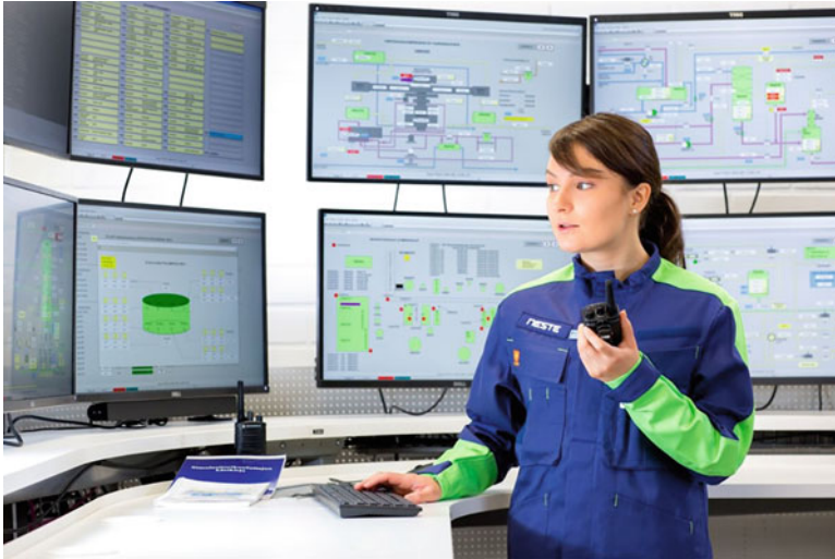
Fig. 1 Simulator training environment replicating the actual workstation of the operator
