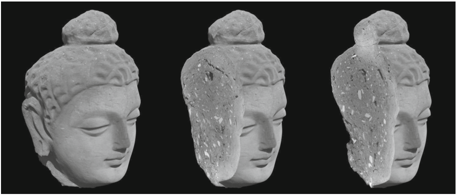
Fig. 5. X-ray CT scanning shows the internal composition of one of the heads and how this type of imaging can show the hidden cross-section of objects without damaging them [17].
