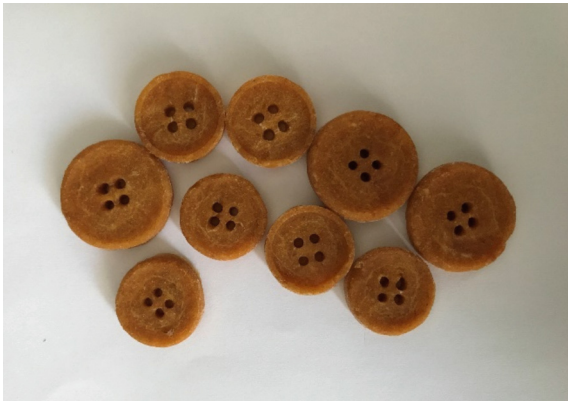
Fig. 7. Prototypes of sustainable and composed buttons produced from organic residues, Source: Author.
