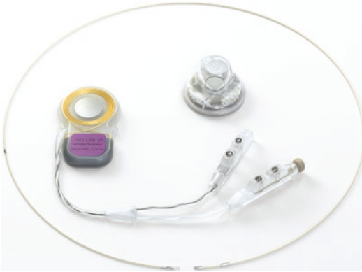
Fig. 19.5 Laryngeal pacemaker system (LP system) consisting of the LP processor (control unit with battery and a coil for inductive transmission), the LP implant (internal electronics in a titanium housing, the receiver inductive coil and connectors) and the active LP electrode for minimal invasive placement in the PCA muscle
