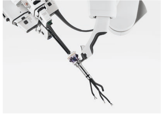
Fig. 32.4 The Single Port (SP) da Vinci system is the latest generation approved for TORS, which provides 3 flexible surgical instruments combined with a flexible endoscope, which are inserted through a single 2.5 cm diameter cannula
