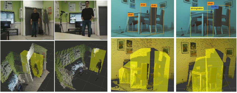
Fig. 8. 3D Object detection using YOLO-v3 and Darknet ROS 3D. Left: shows a person standing and moving in the smart home. Right: shows results in another setting with different furniture.
