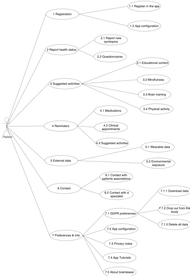
Fig. 5. UML notation of use cases covering key functionalities of the Patient/caregiver app.
