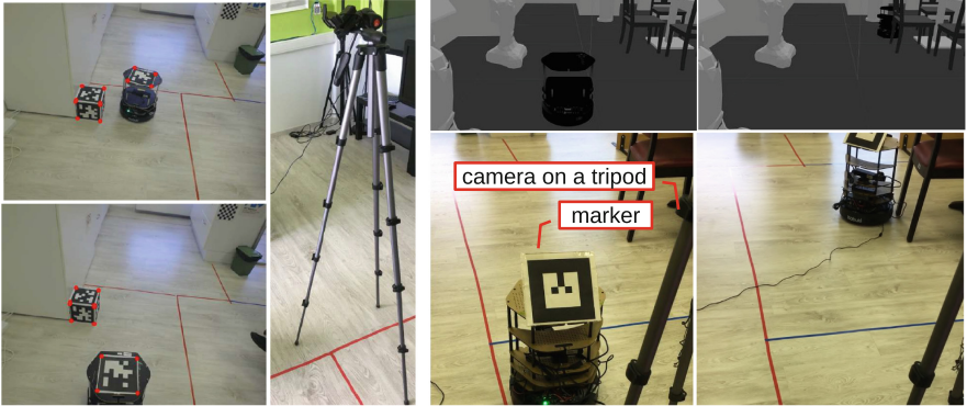
Fig. 4. Left: The trajectory evaluation experiment. Right: Left and right show the Turtlebot at the start and end of the experiment. Top and bottom show the simulated and actual setup.
