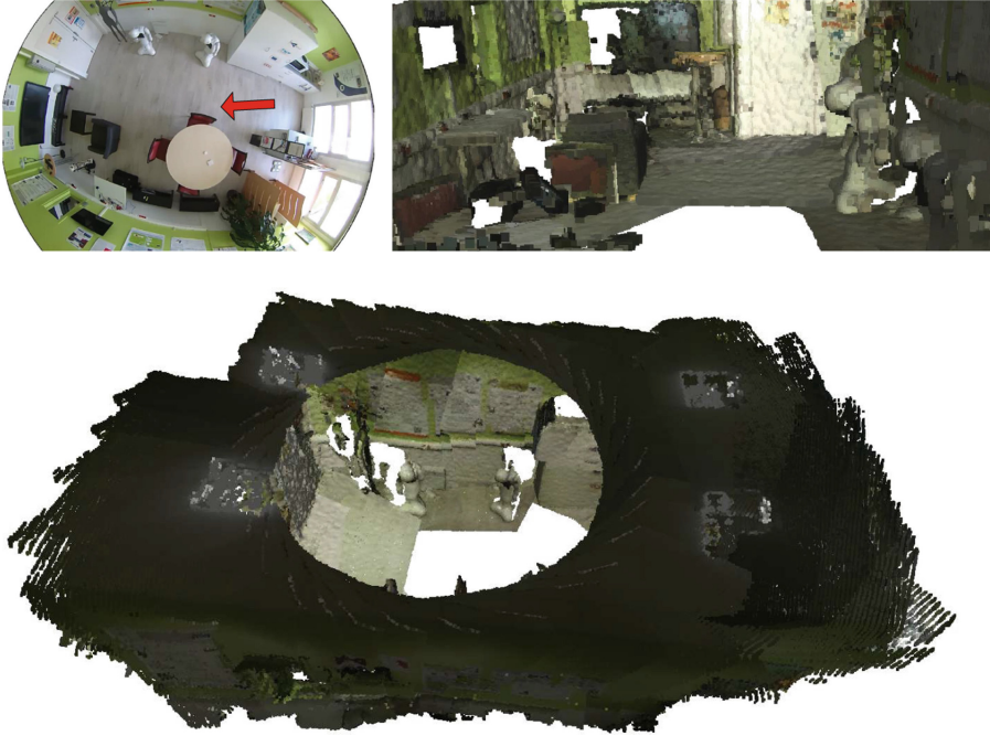
Fig. 2. Top-left: Top panoramic view of the smart home. top-right: Illustration of an area in the reconstructed map (from the view shown by a red arrow in the left image). Bottom: the full reconstructed map (from top view).
