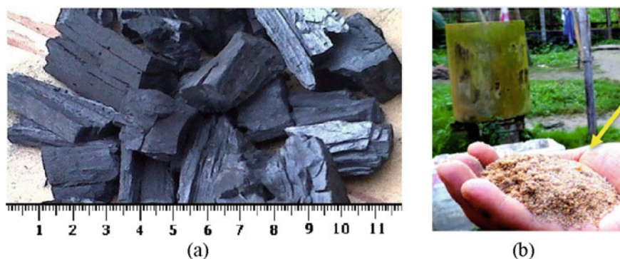
Fig. 13.2 Filtering medium a wooden charcoal pieces as procured and b river sand procured from the filter site
