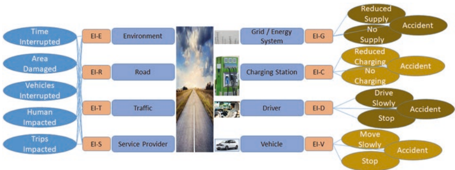
Fig. 10.8 Emergency index analysis for charging station
