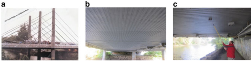
Fig. 5 a 750-ton vessel on bridge. b CFRP configuration. c Impact testing
