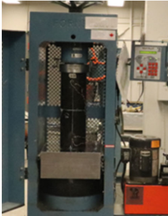
Fig. 1 Testing of CFFTs under compression loading
