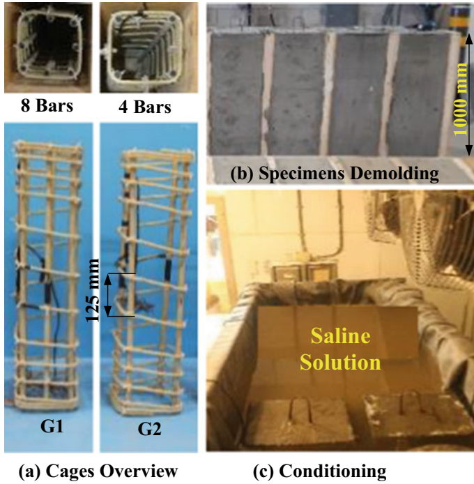
Fig. 2 Specimen preparation and conditioning methods
