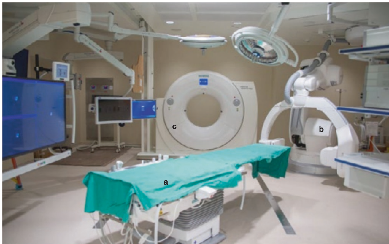
Fig. 53.1 Hybrid room at MD Anderson Cancer Center. (a) Patient table; (b) C-arm fluoroscopy; (c) Computed tomography on rails
