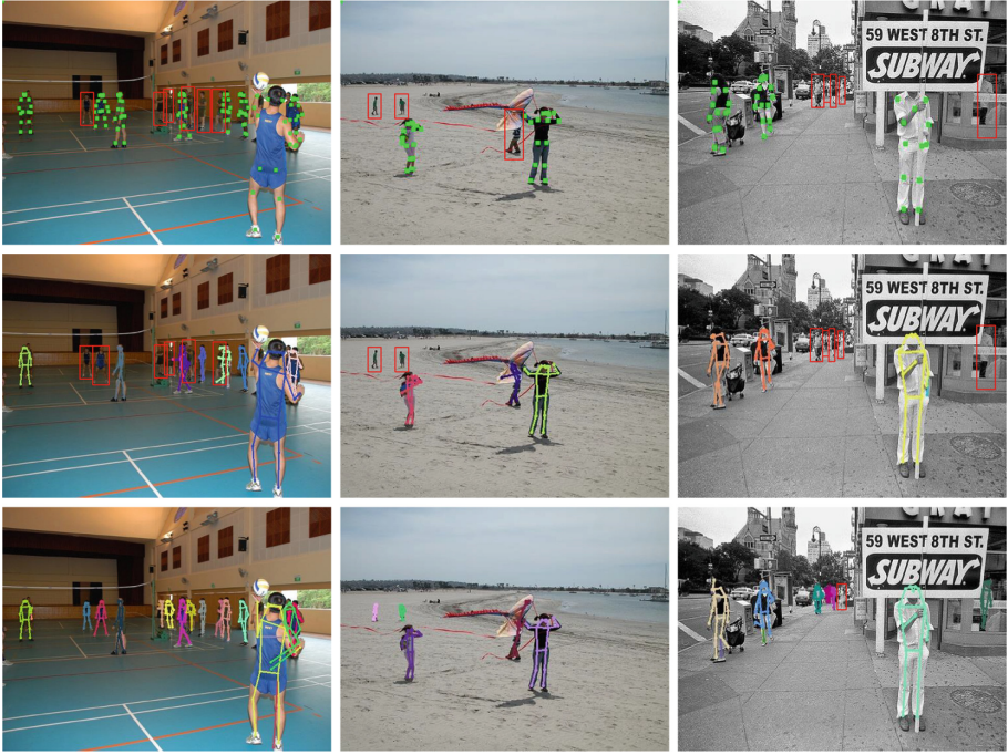
Fig. 4. Top: COCO ground truth keypoints (green). Middle: H_0 predictions when trained on COCO. Bottom: H_0 predictions when trained on Panda-Pose. In all cases, red boxes denote unannotated or undetected persons. (Color figure online)
