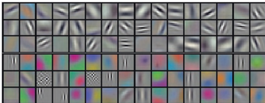
Fig. 6.30 A visualization of the filter weights of the first layer of a VGGNet trained on the ImageNet classification task [29]
