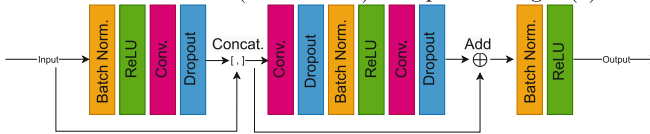
(b) Residual dense-net (RDN) block architecture.
