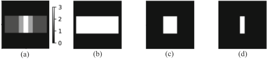
Fig. 3. Decoding of model output a) M_1^{out} into three binary segmentation masks b) M_1^{out} , c) M_2^{out} and d) M_3^{out} , where M_c^{out} denotes the predicted mask with ROI marked by at least c experts.
