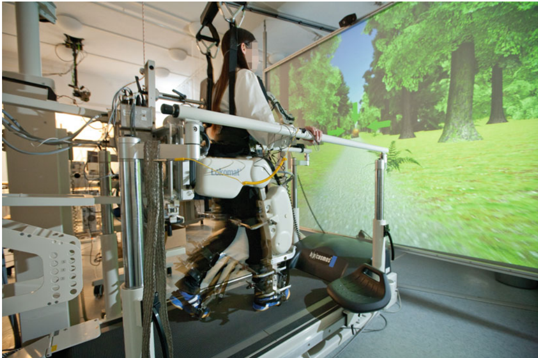
Fig. 29.4 Walking through a virtual environment. Lokomat in combination with a virtual reality back-projection display system
