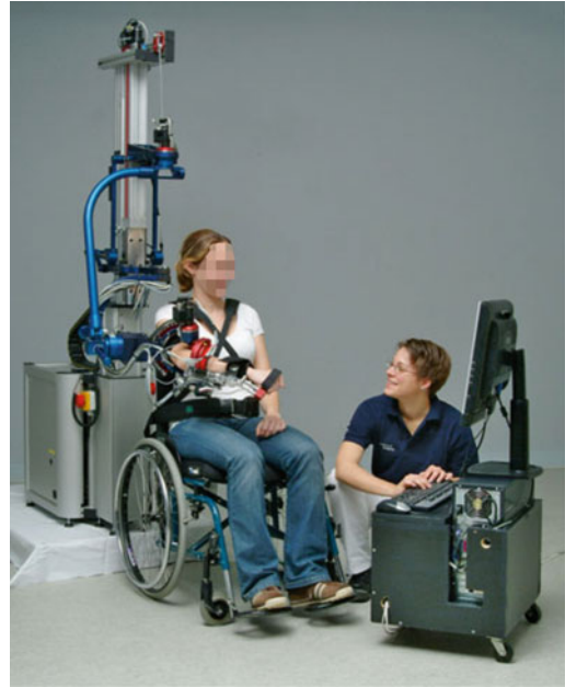
Fig. 27.1 Typical setup for a robot-supported arm therapy system
